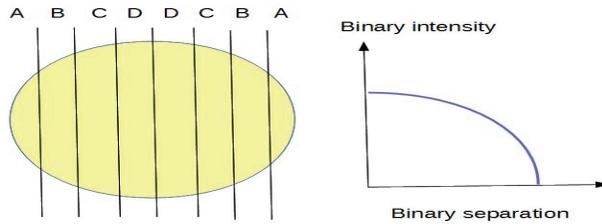
**Figure A. Left** Dissection of a circular disc into binary pairs of increasing separation and decreasing intensity (D is maximum, A is minimum). **Right** Intensity as a function of separation, given by  $\sqrt{1 - (r/R)^2}$ .
