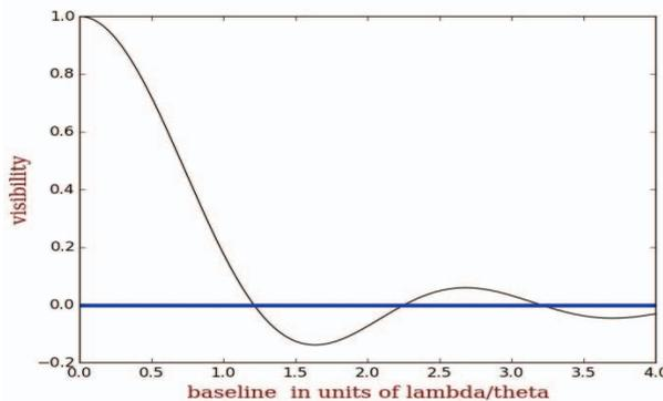
**Figure B.** Visibility as a function of the observing baseline (mirror separation) for a star, modeled as a uniformly illuminated disc of angular diameter  $\Theta$ . This plot is based on the equation given in *Box 2*, and shows that the fringes disappear at a baseline  $b = 1.22 \times \lambda/\Theta$ .
