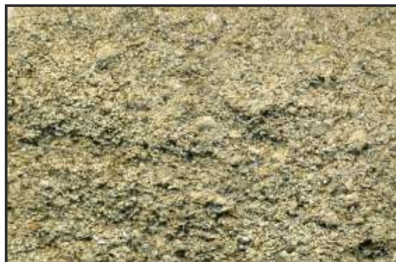
Fig 2. Rock Phosphate after coarse grinding and sizing
