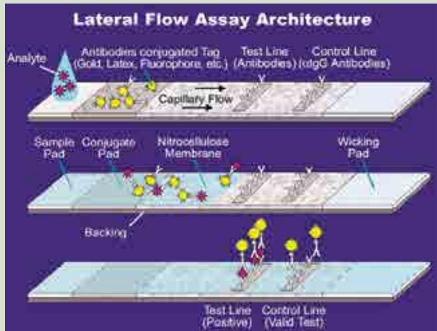
**Fig. 4.** The design of a lateral flow immunoassay.
