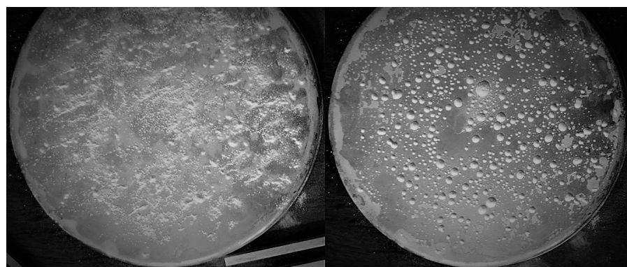
Fig. 2. Mounds of powder making a pattern on a steel plate after touching a tuning fork to it.
